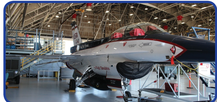
This modified F-16 can simulate the flight characteristics of many other aircraft. Priska Neely/KPCC
